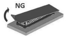
Please do the design of the FPC reinforcement board. When the FPC strength is poor, the connector will break, as shown in the figure.
