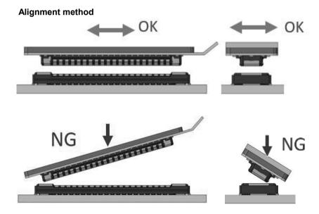
• Insert guide will guide the connector into parallel during insertion and limit its movement from front to back and left to right. Please insert it in parallel according to the picture below.
